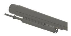
10 - TO REMOVE THE GAS CYLINDER PLUGS USE A PUNCH AND TURN THEM COUNTERCLOCKWISE TO REMOVE
