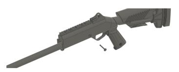
6 - TO REMOVE THE TRIGGER ASSEMBLY, STARTBY PUNCHING OUT THE FIRE CONTROL GROUP RETENTION PIN
