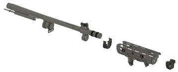
9 - REMOVE THE HAND GUARD AND HAND GUARD BRACKETS FROM THE BARREL
